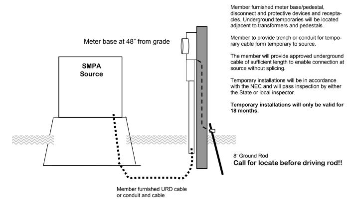
Temporary meter pedestals shall be mounted on **treated 4"x4" wooden post**. The member/electrician will furnish the underground cable, enough cable being provided to reach the transformer/pedestal connection lugs. SMPA will not supply or splice additional cable for the temporary service. The temporary service will be located adjacent to the SMPA power source. Call or see your service planner for locating the temporary service.
