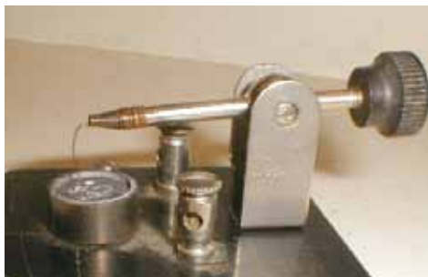
Invented in 1904, the so-called cat's whisker detector was used to rectify the radio signal of crystal radios in the early twentieth century. It was one of the first electronic semiconductor devices ever made.
